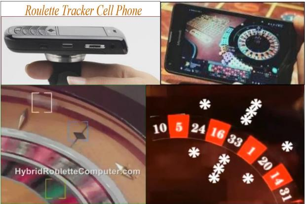
Independent Brackets lock onto and track the spin of the Roulette Ball and the rotation of the wheelhead. A mini-microprocessor determines the most logical fall off point for the roulette ball and what section will be underneath it at point of impact.
